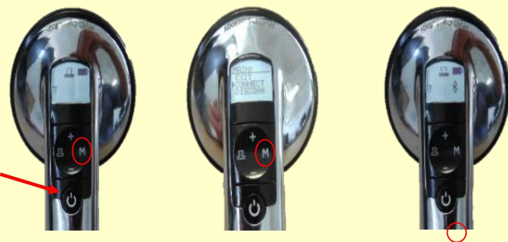
The image shows three sequential close-up views of the stethoscope's control panel. In the first view, a red arrow points to the power button. In the second view, a red circle highlights the 'M' button. In the third view, a red circle highlights the connect button (represented by a Bluetooth symbol).
