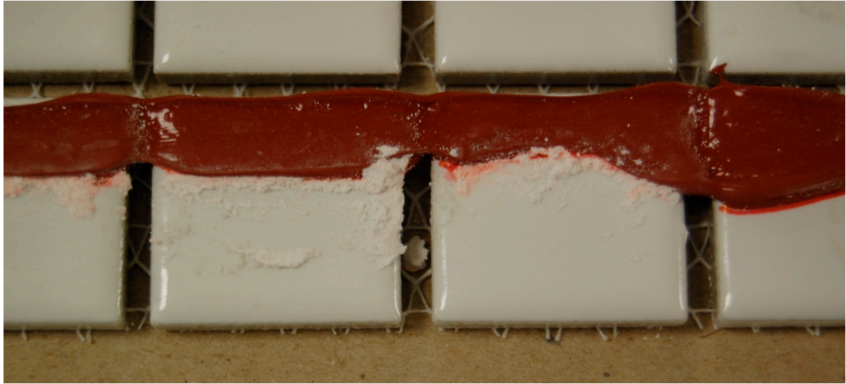
Figure 1: The dental model which has been constructed using ceramic tiles, silicone sealant and grout to emulate teeth, gingiva and calculus respectively.
