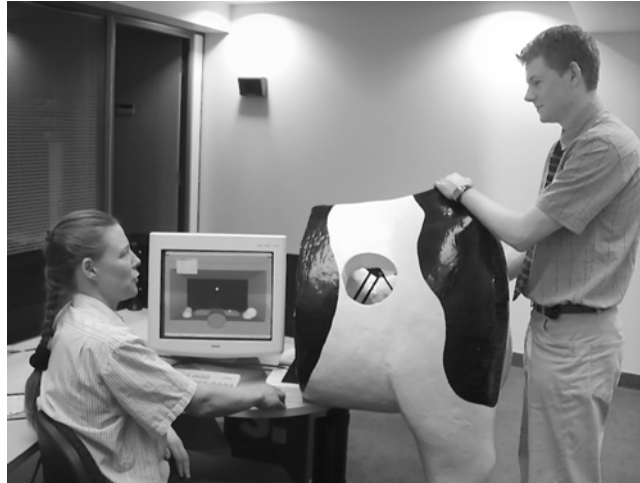
Figure 1: Simulator training. The teacher provides instruction while the student palpates virtual models of the bovine reproductive tract inside the fibreglass cow using a PHANToM.
